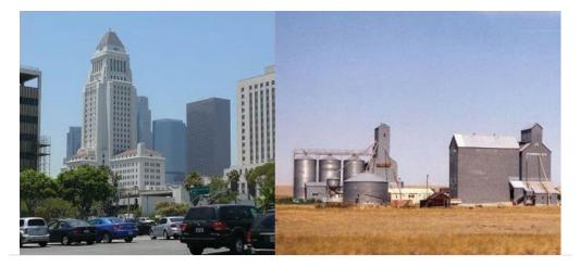
The tall structures shown in Montana are grain elevators used to store grain of local farmers before loading it into railroad cars to be shipped to market.
