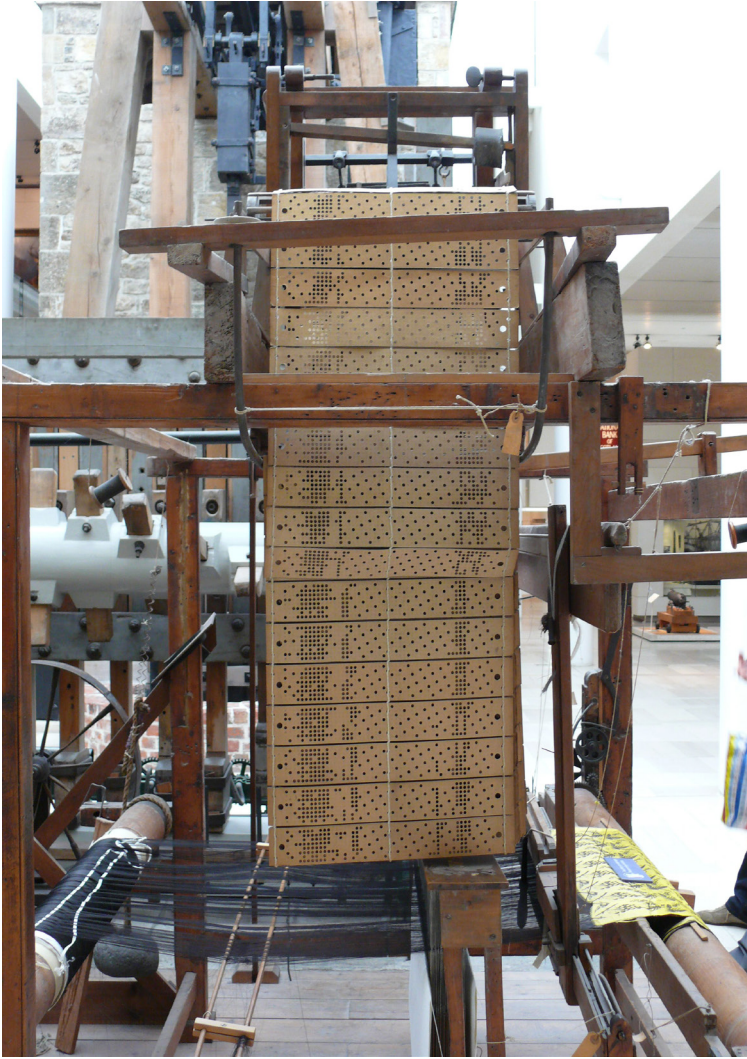
Figure 12.2 Jacquard Loom “NMS Jacquard loom 2.JPG.” by Ad Meskens. This file is licensed under the Creative Commons Attribution 3.0 Unported license.
